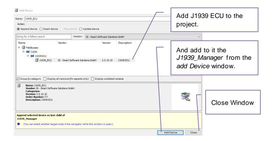
NOTE: DSEM840 has two CAN ports. Within the CODESYS CAN device, set *Network* to 0 for CAN 1, and set *Network* to 1 for CAN 2.
