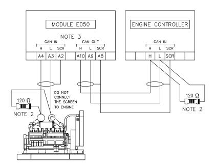
NOTE 2. 120  $\Omega$  Terminating resistor may be required externally, see external equipment manufacturers literature.
