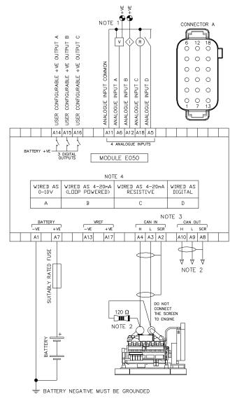
NOTE 1. ANALOGUE INPUT COMMON MUST NOT BE GROUNDED AS IT IS LNIKED INTERNALLY TO TERMINAL A1.
